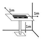
For best operation, the receiver should be at least 1m above the ground and 1m away from a wall or metal surface to minimise reflections. The transmitter should also be at least 1m away from a wall or metal surface to minimise reflections. The transmitter should also be at least 1m away from the receiver. Keep antennas away from noise source such as motors, automobiles, neon light as well as large metal objects.
