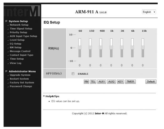
The EQ of every input can be set individually. Each input is set by selecting the respective channel button. Default value is 0 for each band. 20 Steps can be set from -10 to +10. High pass filter (65Hz) can be set for each input.
